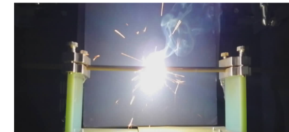
图 11 球墨铸铁电极材料故障电弧现象 Fig. 11 Arc fault phenomenon of ductile iron electrode
